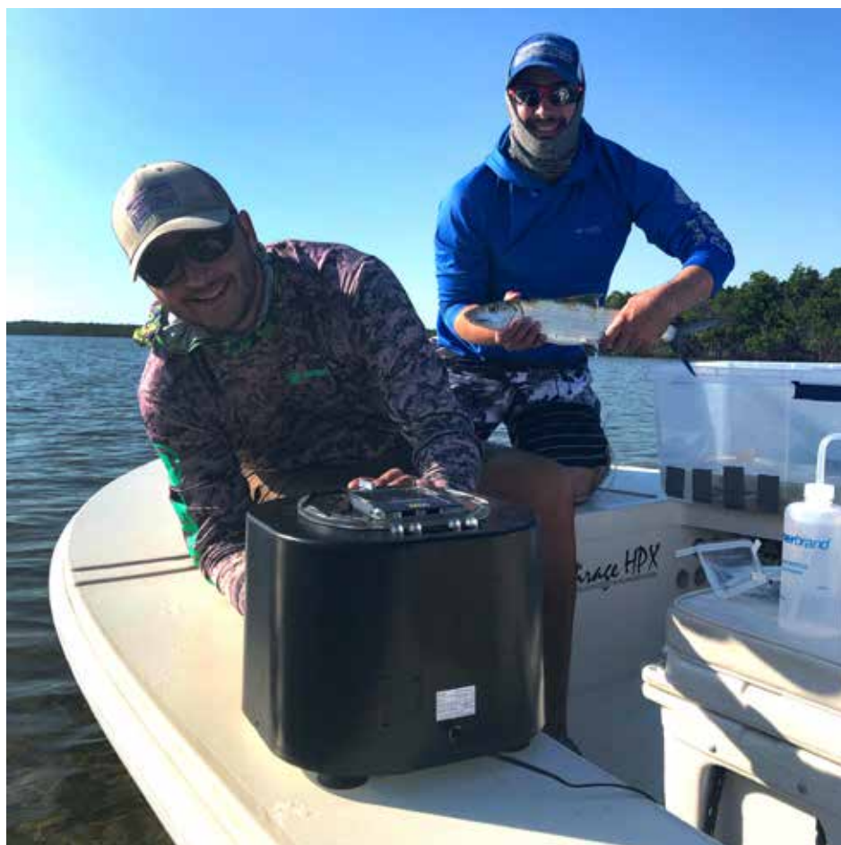
Bonefish samples are taken and processed on the water. Here Nick Castillo uses a portable centrifuge to spin blood taken from a Key Largo bonefish. The plasma is separated from the blood cells and the plasma is then analyzed for pharmaceuticals. Photo: Capt. Brett Greco
